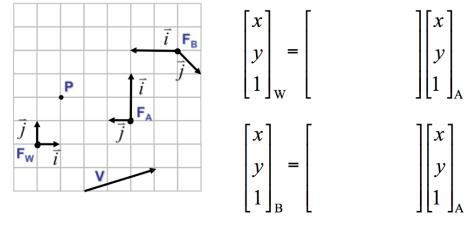
(a) Express point P in each of the three coordinate frames. F<sub>W</sub>, F<sub>A</sub>, F<sub>B</sub>.
