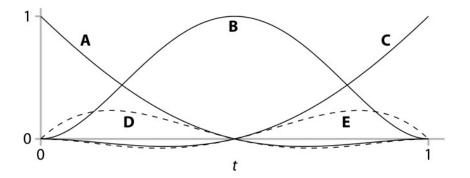
(a) Which of the five control points (arbitrarily labeled A through E in the plot) will the curve pass through, and for what values of t?
